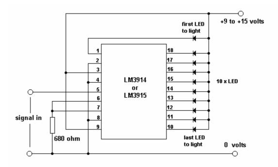
One application of the bargraph can be seen on the front of Hi-Fi amplifiers, where an array of LED's indicates audio levels. As the signal increases, the LEDs come on in ascending order.
